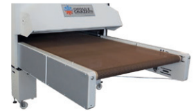
single belt conveyor
